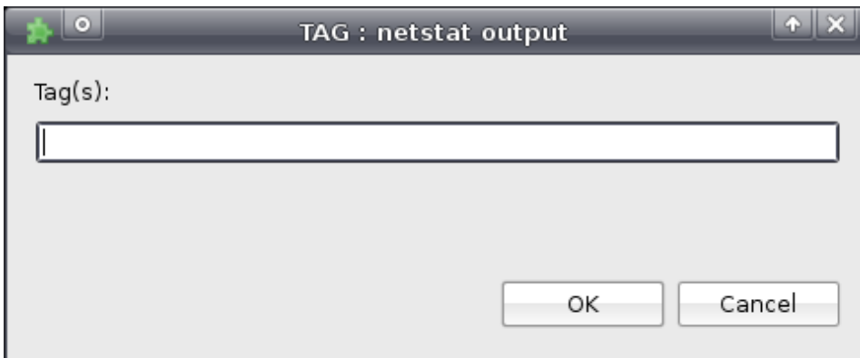
Figure 36. The dialog invoked after selecting a data set or a tool and pressing ALT-T. The tag will be used for sorting the files.
