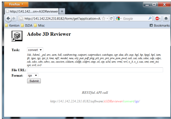
Figure 3. The form presented to a user after clicking on a software icon within the browser view of a software server. From this form the user can select a task to perform, select an input file, select an output format (which may be the same as the input format), and submit the task to be executed. To emphasize the available RESTful API access to the software functionality we display the API call below and update it in real time as the user makes selections. The user can achieve the same effect of pressing the “submit” button by simply accessing the shown RESTful API URL.
