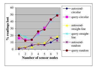
Figure 1 Percentage of readings lost in 'autosend' and 'query' data collection schemes
