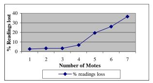
Figure 2. Percentage of readings lost as a function of number of motes in 'other' network
