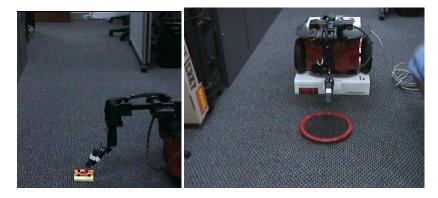
Figure 4: Robotic system for BTF data acquisition. Object BTF modeling (left) for ATR applications and clutter BTF modeling (right) for scene understanding and simulation applications.
