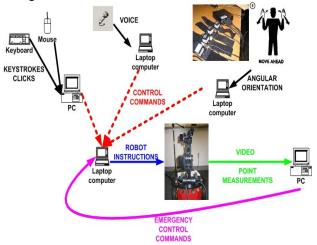
Figure 1: An overview of a system for remote robot control using sound, gesture and human-computer interface inputs.
