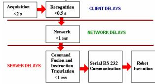
Figure 6: Delays occurring between the time a command is given and executed by robot
